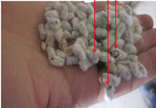
Figure 1 - Mechanical or physical damages (wounds, Scratches and fractures of the seed coat) caused during ginning process at the ginning factory.
