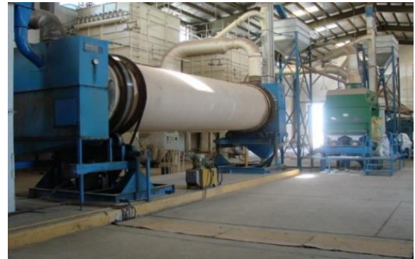
Figure 7 - View of the interior of the Kashmar cotton seed delinting factory, one of four factories located in Iran that works with the dilute sulfuric acid and heat method.
