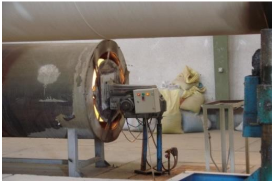
Figure 7 - View of the interior of the Kashmar cotton seed delinting factory, one of four factories located in Iran that works with the dilute sulfuric acid and heat method.
