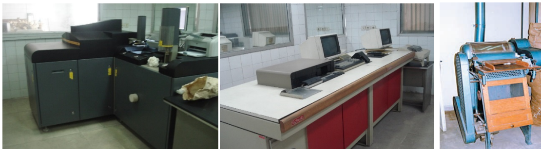
Figure 11- Laboratory small scale gin equipment used for seed cotton samples ginning (right) and High Volume Instrument (HVI) equipment (middle and left) used for cotton varieties fiber quality characteristics measurement.
