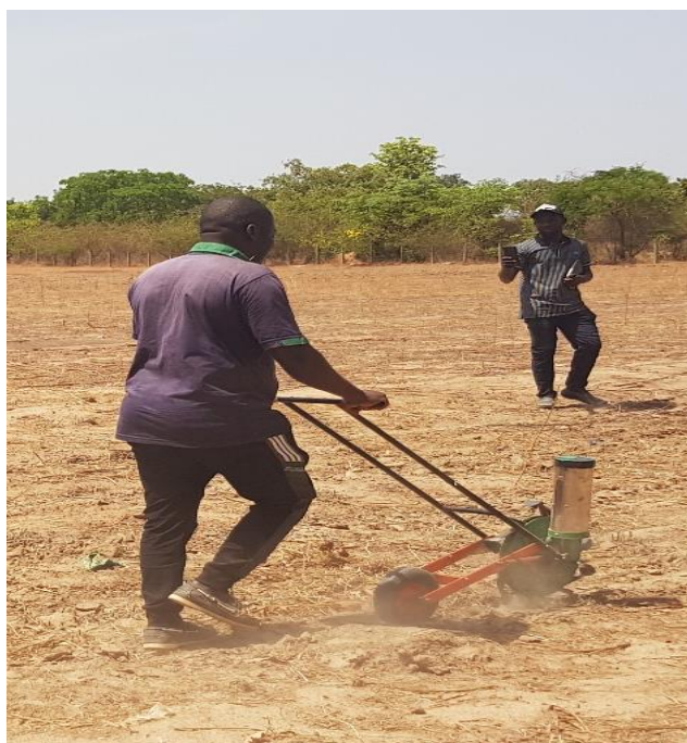
Figure 5: Hand-operated wheeled seeder
